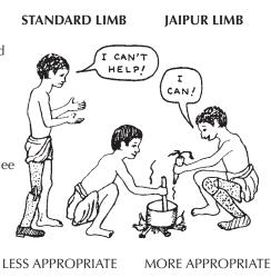
The 'Jaipur limb' was designed for the needs of villagers in India. It has a knee with a joint that bends all the way. The foot piece is made mostly of rubber and is very flexible, allowing the person to squat. It is the color and shape (including toes) of a normal foot. It is waterproof, so that people can work in water or rice fields without harming it. The leg is low cost and quick to fit.
